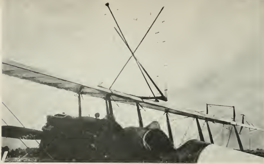
TWENTY-FIVE YEARS AGO, THE CUMBERSOME RIG ON THIS BIPLANE'S TOP WING WAS DEVELOPED AS A RADIO DIRECTION FINDING LOOP ANTENNA.
