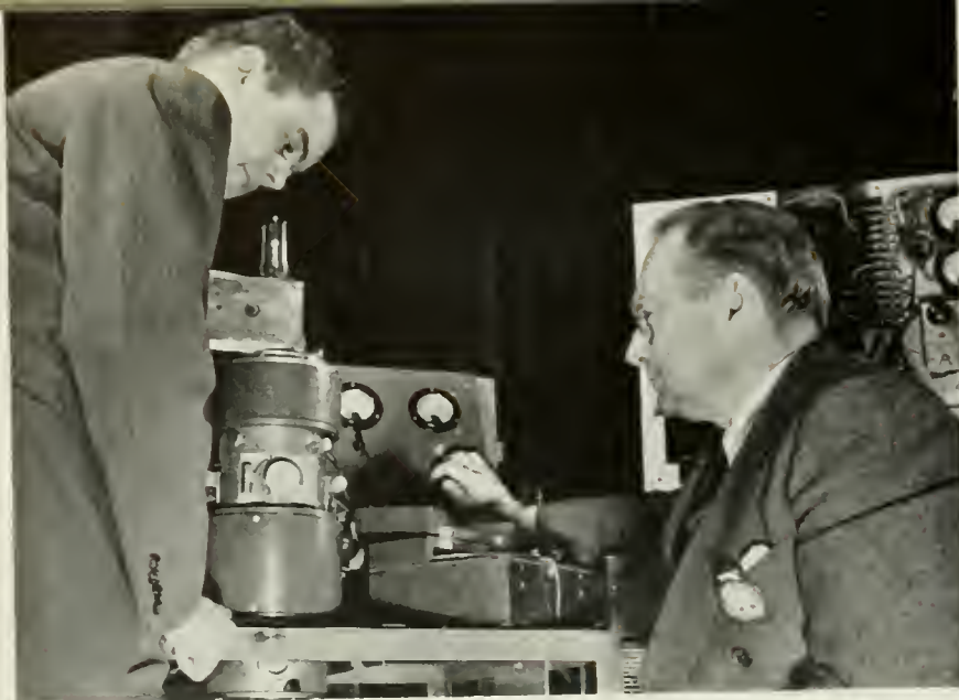
DR. JAMES HILLIER (LEFT) AND DR. V. K. ZWORYKIN OPERATING THE ELECTRON MICRO-ANALYZER DESIGNED TO GIVE AN ELEMENTAL CHEMICAL ANALYSIS OF ULTRA-MICROSCOPIC PARTICLES OF MATTER.
