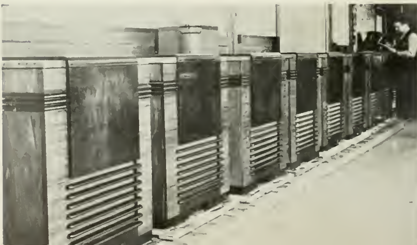
PRE-WAR TELEVISION RECEIVERS ROLLING OFF THE FINAL ASSEMBLY LINE AT THE CAMDEN, N. J., PLANT OF THE RCA VICTOR DIVISION. THEY WERE THE LARGEST MODELS, TRK-12, BUILT BY RCA.
