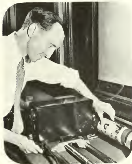
BELOW: HIGH-SPEED MULTIPLEX RADIO-TELEGRAPH PRINTERS TRANSMIT MESSAGES ACROSS THE SEAS AT THE RATE OF HUNDREDS OF WORDS A MINUTE.
